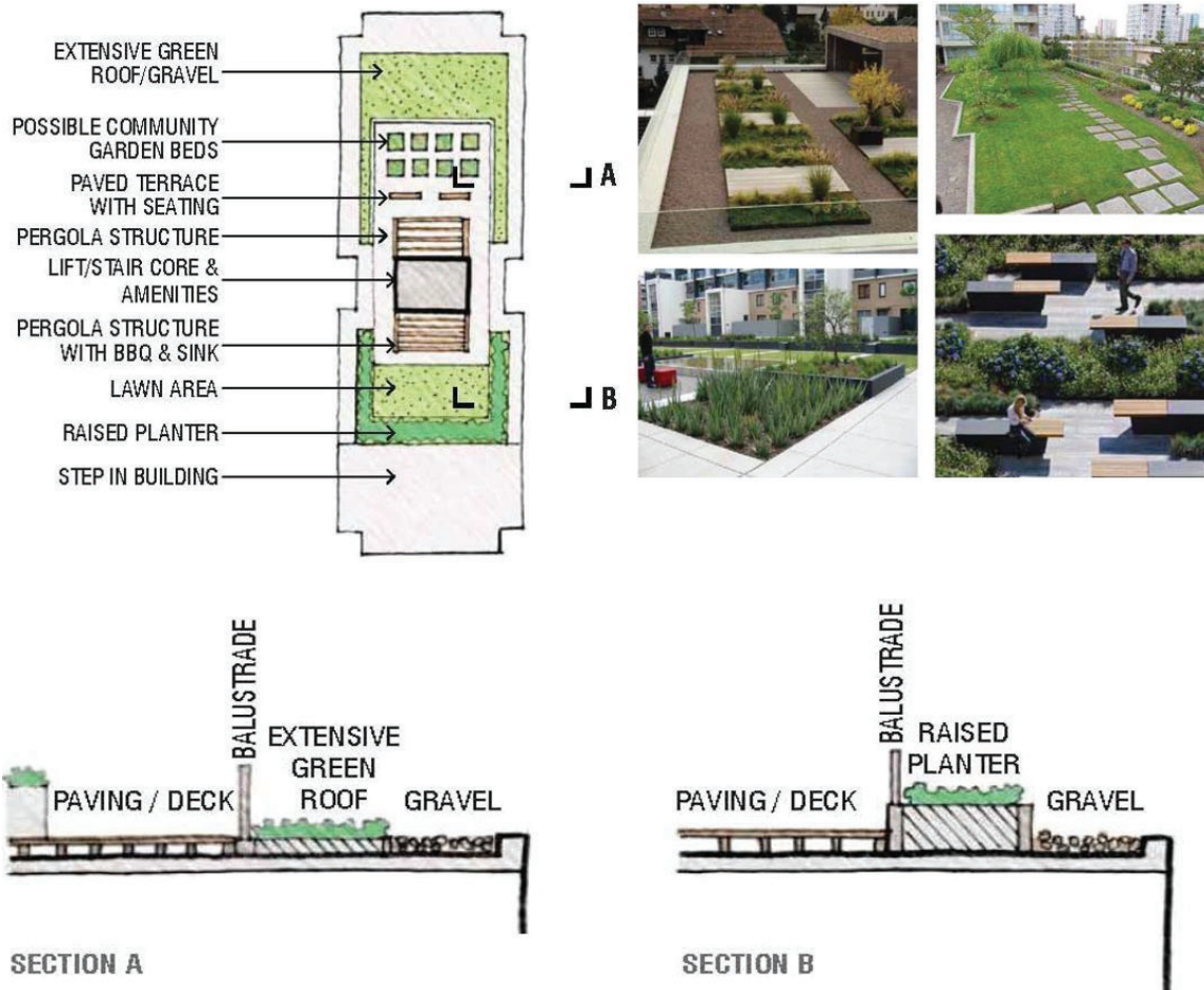
Figure 25 (b): Roof Terraces – Details
